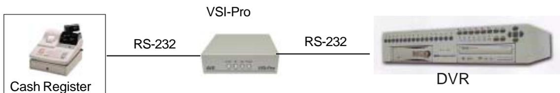
The AVE line of IF ECR Interfaces, Parallel to Serial, USB & TCP/IP adapters along with many other special converters and adapters output data in the formatted RS-232 protocol. Many DVRs can receive this data directly without the use of a VSI-Pro.
